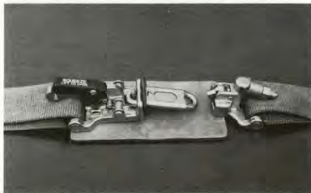
The HBU-12/A automatic belt buckle hardware and gold key is shown separated as before hookup (left) and after automatic disconnection (right). The surest way to be certain the belt is locked is to press down on the handle after the belt is connected, then pull up on the handle without depressing the black top of the handle.
