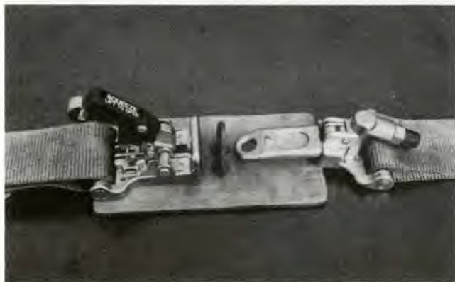
The HBU-12/A automatic belt buckle hardware and gold key is shown separated as before hookup (left) and after automatic disconnection (right). The surest way to be certain the belt is locked is to press down on the handle after the belt is connected, then pull up on the handle without depressing the black top of the handle.
